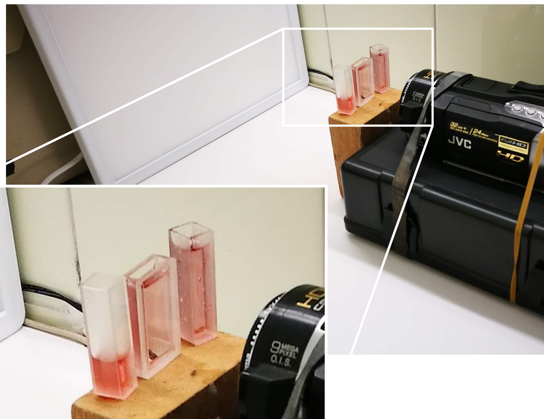
Figure 3: Optical setup. The arrangement of the LED backlight, photo spectroscopic quartz cuvettes and the video camera is shown; inset shows a zoom on the cuvettes.
